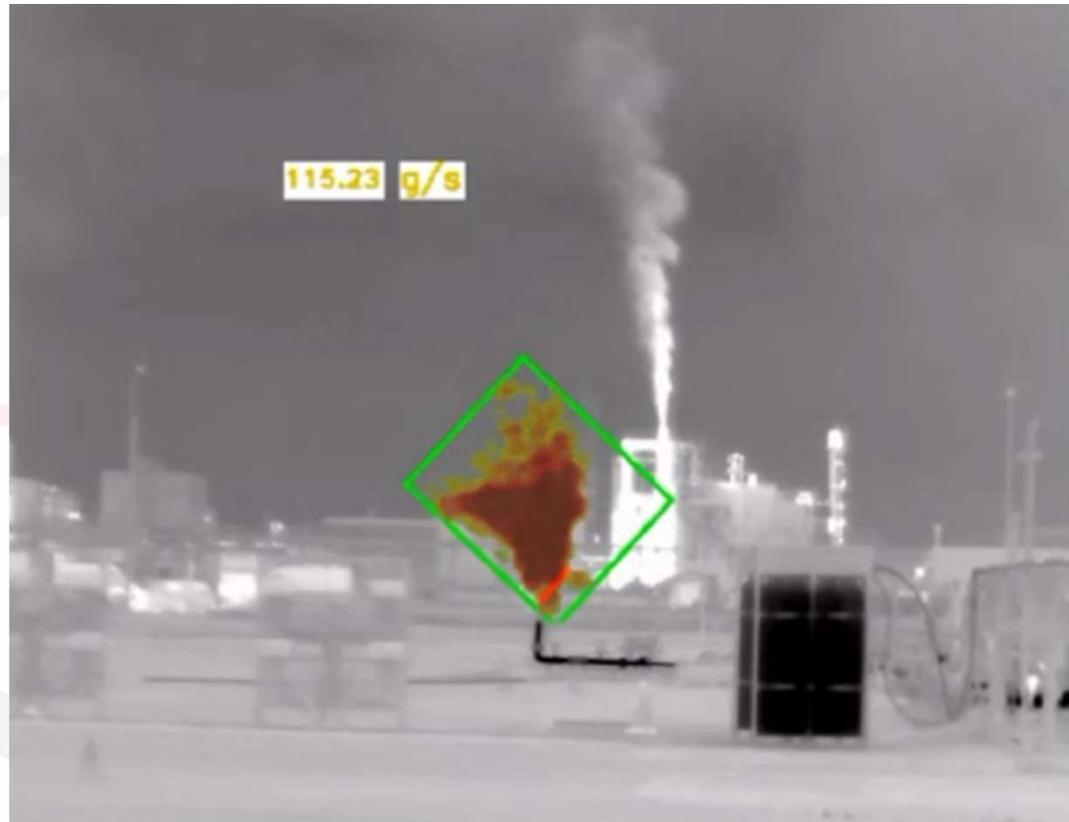
Leak flow rate 100 gr/sec CH<sub>4</sub> at 100m
