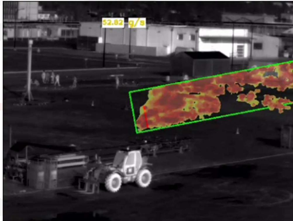
Leak flow rate 50 gr/sec (180 kg/h) of CH<sub>4</sub> at 100m
