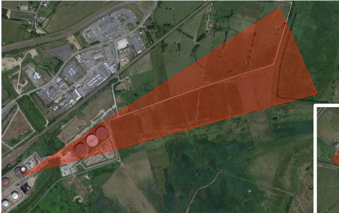
Multiple tanks roof monitoring using 1 or 2 cameras
