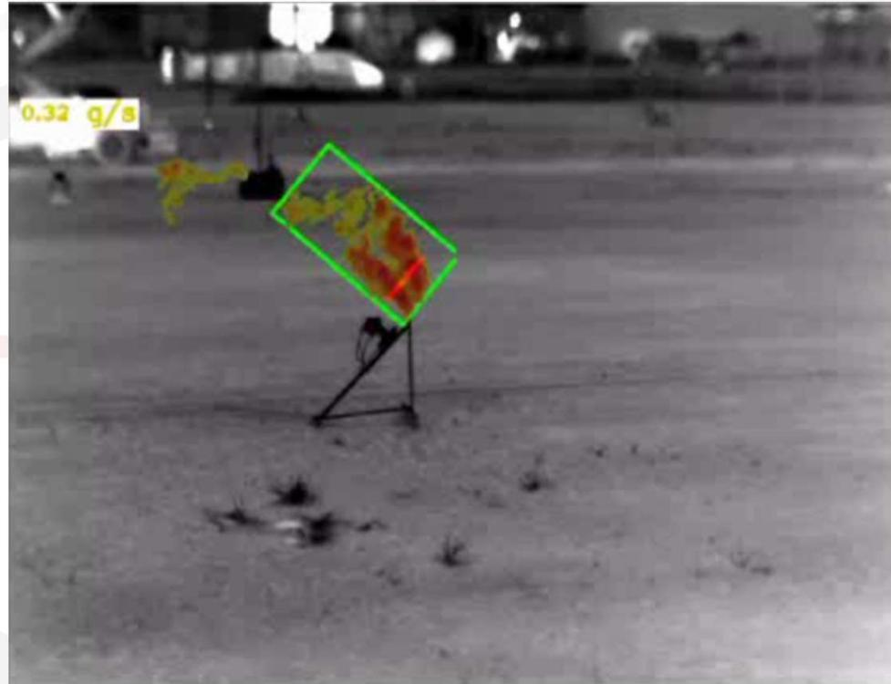
Leak flow rate 0,32 gr/sec (1,15 kg/h) of CH<sub>4</sub> at 50m
