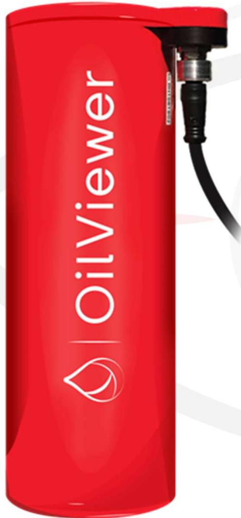
Specifically designed for real time detection of oil spills on water and ground surfaces in continuous automatic mode. It detects the specific fluorescence of oil caused by its exposure to certain UV light emissions, while not reacting to other materials that may appear in the observation area, in order to reduce false alarms.
