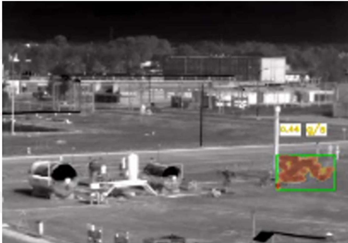
Leak flow rate 0,45 gr/sec CH<sub>4</sub> at 100m
